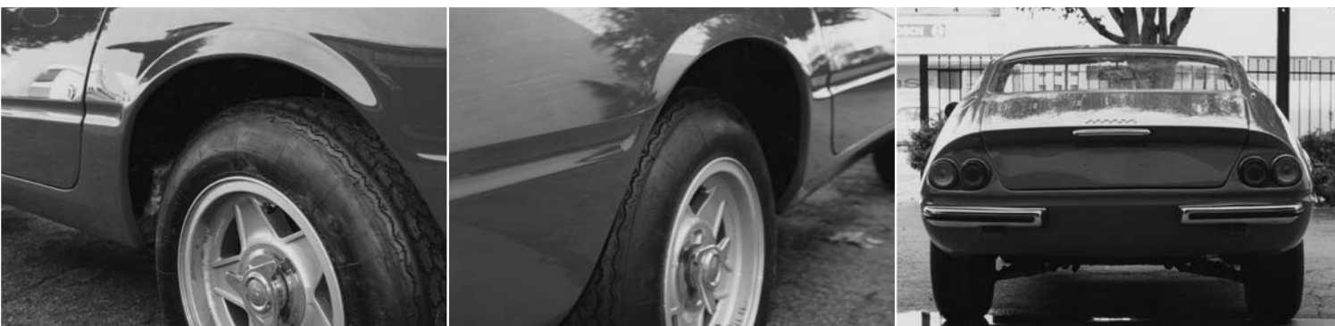
The Daytona's left and right sides of the body were not very symmetrical when we received the car. Note the vast difference of rear fender wheel well openings relationship with each wheel/tire assembly.
